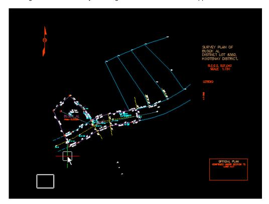
Next you will be prompted to input the X scale factor for the block. Because this is a metric drawing scaled to 1:750 I will enter 750:
