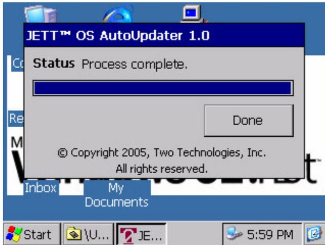
When you click the "DONE" button, you will see the following message displayed. At this point, remove the battery, wait 5 seconds, replace the battery, and power the unit on.
