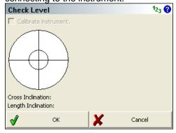
17. Switch back to the **Model and Communication** screen. Press the **Connect to Instrument** button and if you successfully connect you will see a green check mark on the Connect to Instrument button, and the Check Level screen will appear. Have fun!
