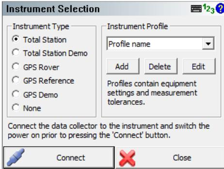
Depending on the type of instrument you are connecting with select Total Station, GPS Rover or GPS Reference (Base)
