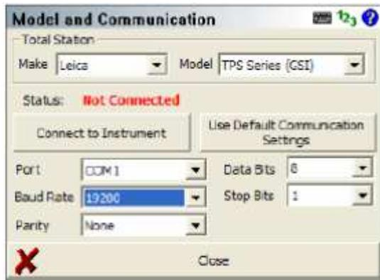
If you are using a Leica Prism, use the settings below as a guide. "Set Instrument to Zero" commands FieldGenius or EVR to set the prism type to "Circular" and allows the software to apply the offset.
